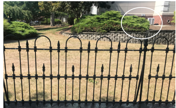
Screening equipment with landscaping and placing units far back from the street helps preserve the historic streetscape, even at modern buildings. A concealed condenser unit is circled.
